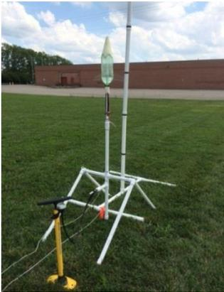
3. Measure and mark three observation sites at least 100 feet away from the launcher and 120° apart relative to the launcher.
