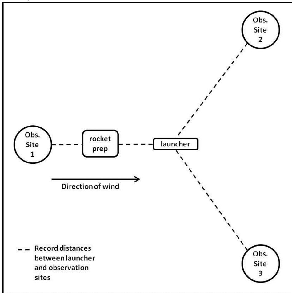
4. Setup rocket preparation area using water source with graduated cylinder
